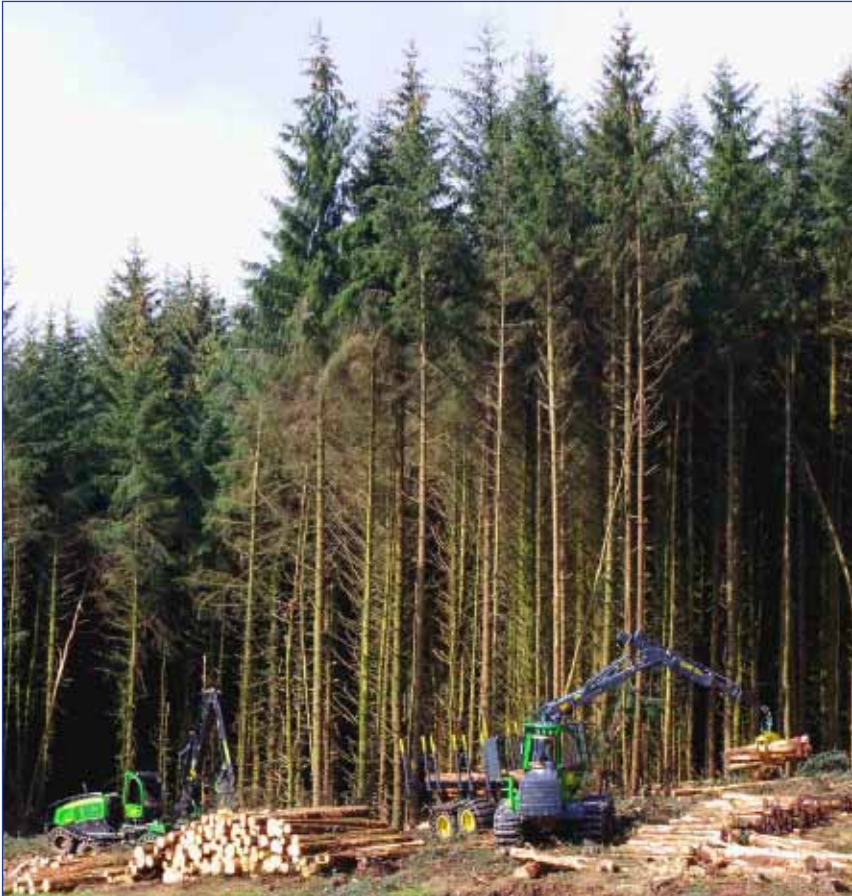
Conifer plantation being felled for timber, using a harvester at left, and the forwarder at right which carries logs to transport trucks.
